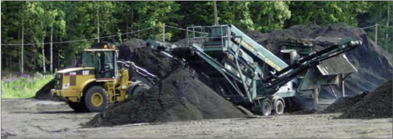
Figure 12. A crusher breaking up self-hardened ash at Borås, Sweden.
