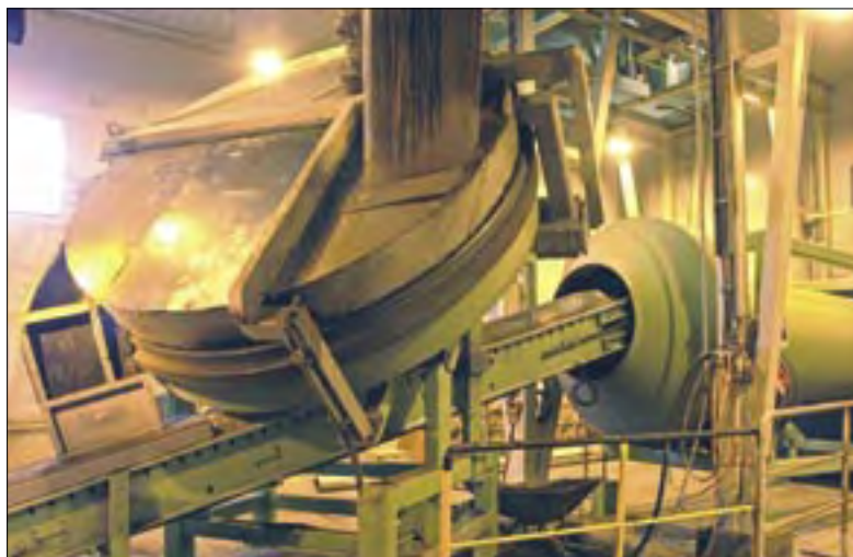
Figure 15. Granulation unit comprising plate granulator and drum type post-granulator at Enotuhka Oy, Stora Enso's Enocell pulp and paper plant. Enocell owns the equipment, Enotuhka Oy is responsible for its operation and Astera Ky designed and manufactured the post-granulation unit. The volume of granulation is 4 000-5 000 tonnes annually, but production capacity is much greater. Photo Samuli Rinne, VTT Processes.
